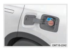
Step 3: Turn the fuel filler door counterclockwise;
