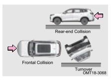
The front seat side airbag, curtain side airbag (if equipped) and center airbag (if equipped) may not deploy if the vehicle is subjected to a front or rear collision, turnover or low speed side collision.
