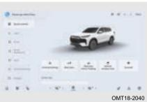
When the vehicle is powered on, click " = " button through Audio System - Settings - Quick Control to turn on/off passenger side window OFF function
