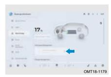
With vehicle powered on, turn on/off external discharging function under charging/discharging management screen of head unit system. Before unplugging the discharging gun, it is necessary to turn External Discharge to OFF.
