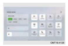
When the vehicle is powered on. When the vehicle is stationary and the gear position is in D/N/R, parking radar system turns on automatically; When parking radar system turns on and the gear position is in D/N (" \( \frac{1}{2} \) " button is highlighted), click " \( \frac{1}{2} \) " button on control center to turn on/off parking radar system manually.
