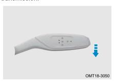
Fully depress brake pedal and shift the shift lever to D: Release the brake manually parking automatically and release the brake pedal, and then drive the vehicle slowly.
