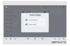
When the vehicle is powered on, turn on Forget reminder through Audio System - Settings - Connect.
