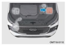
Step 3: Remove front compartment fuse box cover, refer to fuse box location diagram at fuse box upper cover, pull BMS fuse out by a fuse remover and disconnect the BMS module power.
