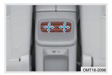
Move the second row outlet adjustment lever up, down, left or right by hand to adjust direction of airflow.
