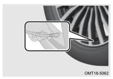
Tighten the junction valve of the automatic inflation tire repair liquid to the tire valve;
