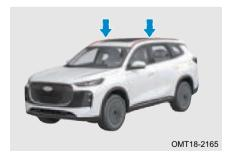
Roof carrier is used for loading cargo. Be sure that the total weight of the loading cargo on the carrier or loading tool (such as luggage compartment, cross rod)
