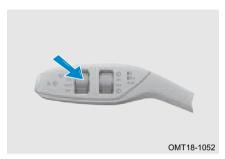
When the vehicle is powered on, pull wiper switch towards the steering wheel and release it to flash the high beam lights once. At the same time, high beam lights indicator in instrument cluster flashes once.
