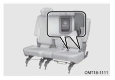
The rear outside seats are equipped with ISOFIX / i-Size anchorages. The anchorage locations are identified by a marking (see illustration) located on the seat back, directly above the associated anchorages.
