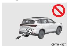
When washing vehicle, use a soft cloth or water (low water pressure) to wash off foreign matter such as snow, mud, and dust on the surface of radar sensor.
