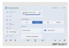
When the vehicle is powered on, slide and adjust the Opening height setting for tailgate through Audio System - Settings - Vehicle Settings.
