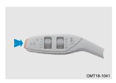
Spray mode: Shortly press the left button of wiper switch and hold, the front washer sprays water, and front wiper operates simultaneously. Front washer will stop operating when the switch is released, the wiper will wipe 3 cycles at low speed, and operate one cycle then stop after a few seconds.
