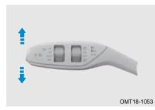
When the vehicle is powered on, dial wiper switch upward, right turn signal light is turned on; Dial downward, left turn signal light is turned on.
