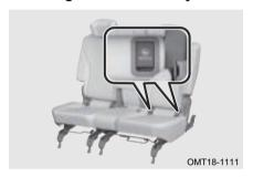
Step 1: Locate the ISOFIX anchorage; Please adjust the front and rear travel of the second row seat to the last position.
