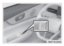
Press " switch to turn on/off the passenger side window OFF function.
