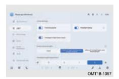
When the vehicle is powered on, set headlight height adjustment (level 0/ level 1/level 2/level 3) through Audio System - Settings - Light.
