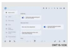
When the vehicle is powered on, turn on automatic folding of exterior mirrors through Audio System - Settings - Quick Control; In disarming/arming, outside rear view mirror will be folded/unfolded automatically.
