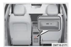
Rear USB is located at the rear of center armrest box (as shown in the illustration).
