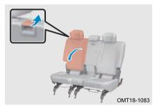
Pull up EASY ENTRY operation handle at upper part of seatback, fold the second row seatback and slide the second row seat to foremost position to easy access to third row seat.
