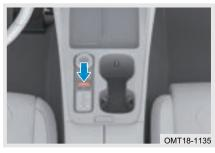
With vehicle in READY state, dial knob (EV/HEV) to switch the power mode; The corresponding mode indicator on instrument cluster comes on to prompt you that power mode is switched successfully.
