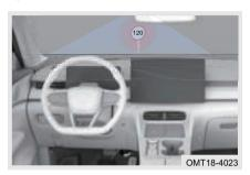
After SLA detects speed limit sign information on road ahead and combines the information with speed limit information of navigation system, "
