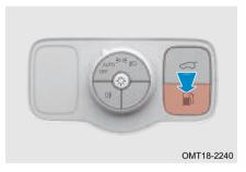
Step 1: Switch vehicle to power off state, long press " " button and instrument cluster displays "It is ready to refuel, please refuel" message, and fuel tank cap is unlocked after pressure relief is completed;
