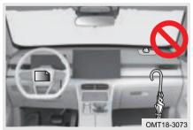
Do not attach anything to or lean anything against the areas such as the instrument panel, steering wheel and lower portion of the instrument panel. These items may be thrown out when driver frontal airbag or front passenger frontal airbag deploys.
