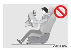
There should be no objects on deployment path of airbag. It is forbidden to place anything (such as mobile phone, etc.) between the occupant and the airbag. Never fix or place any object on or near the airbag cover. If there is an object between occupant and airbag, the airbag may not deploy according to designed path, or the airbag may push object into occupant's body, causing serious injury or even death.
