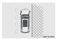
If there is no curb on the roadside, turn the steering wheel hard right to prevent the vehicle driving into the center of the road or sliding down the slope. Turn the steering wheel to the side of the road, so the vehicle is facing away from the center of the road when moving, then apply the parking brake.
