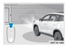
ON: Turn vehicle power to OFF mode, turn on headlight automatic mode before stopping. When the vehicle is in a dim environment, press unlock button on smart key, low beam lights will come on for tens of seconds. Press unlock button to activate it again.
