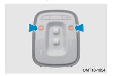
Touch the front left/right dome light, the front dome light on corresponding side comes on.
