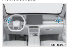
Move left/right side outlet adjustment lever up and down, left and right by hand to adjust direction of airflow.
