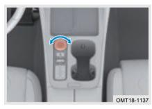
With vehicle in READY state, turn the drive mode knob to cycle through the drive modes; The corresponding mode indicator on instrument cluster comes on to prompt you that drive mode is switched successfully.
