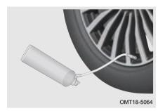
5. After the automatic inflation tire repair liquid is filled, close the valve counterclockwise and screw out the junction valve. Then immediately drive for 10 km or more to complete the repair. Please go to the authorized service station or professional tire repair shop for repair and replace as soon as possible.
