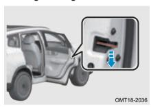
Open the door, insert the mechanical key into the lock cylinder, and move the lock button downwards to lock the door.
