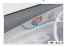
With vehicle in unlocked state, pull door inside handle directly to open doors.
