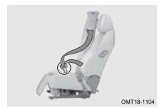
Check seat belts regularly for cuts, fraying, loose and stretched belt (such as after a traffic accident). If the belt is damaged, please contact authorized service station for inspection and repair immediately.
