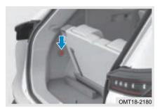
The rear backup power supply is located on the left side of luggage compartment (as shown in the illustration).
