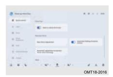
When the vehicle is powered on, and turn on Near to unlock, far to lock through Audio System - Settings - Quick Control.
