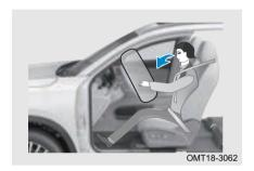
In an event of a severe frontal collision, driver frontal airbag, front passenger frontal airbag and driver knee airbag (if equipped) work together with seat belts to help reduce injuries to the head or chest of driver and front passenger by hitting the caused interior component. (Front passenger frontal airbag may be activated even if there is no occupant in the front passenger seat).
