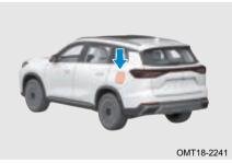
Step 2: After fuel tank cap is unlocked, push fuel tank cap, it will pop up;
