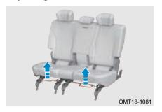
Pull up the seat adjusting grip, move the seat back and forth to desired position, and release grip to adjust the seat position.
