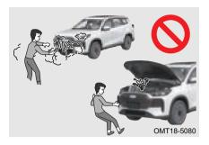
If there is steam or coolant spraying out, it indicates that pressure in cooling system is very high. To avoid personal injury, keep the hood closed until there is no steam spraying out.
