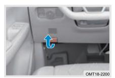
Step 1: The hood will spring up slightly when the hood release lever is pulled twice;
