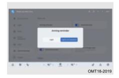
When the vehicle is powered on, and set Arming reminder (Light/Lights and Speakers) through Audio System - Settings - Vehicle Settings.
