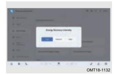
With vehicle in READY state, set energy recovery intensity (low/medium/high) through Audio System - Settings - New Energy.
