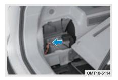
Step 2: Open the tail door and remove the left trunk guard Plate, disconnect battery (12 volts) negative cable;
