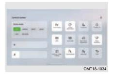
When the vehicle is powered on, click "  $\Box$  " button on the control center to fold/unfold outside rear view mirror.
