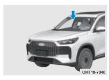
The microwave window is located at right side on back of front windshield inside rear view mirror where is for wireless RF signal transmission and installation of automotive electronic identification.
