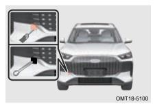
Use a screwdriver with its tip wrapped with tape to remove the towing eyelet hole cover;
