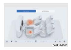
Method 1: After starting the vehicle, click second row seat heating button by air conditioning display screen - seat - heating, it is 3-level heating (3 indicators on). Each time the switch is clicked, the heating level is lowered one level. Click it the fourth time to turn off the seat heating.
