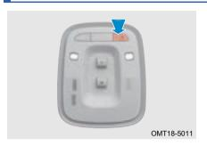
ECALL is a kind of emergency call function. When vehicle is involved in a certain level of impact (airbag when driver inflated) or passenger is in an emergency and rescue is required, emergency information can be sent to service center bν operating button manually, then the center will track vehicle location and promptly offer rescue according to received information.
