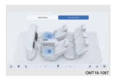
After vehicle starts, click " button through Audio System - Seat Control Screen - Seat Ventilation to turn on the seat ventilation function and switch among level 3/level 2/level 1/OFF circularly.
