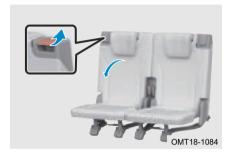
Pull seatback adjustment lever upward, and slowly lower the seatback with your hand, then seatback can be folded.
