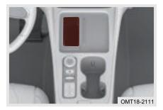
Turn vehicle power to non-OFF mode and the wireless charging function is enabled, when the wireless charging starts to work after putting the mobile phone in wireless charging sensing area, the audio system updates the charging icon in real-time based on the charging status. If the charging fails, the charging icon turns red.
