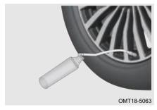
4. Turn the red valve clockwise and place the bottle upside down to start inflating the tire;
