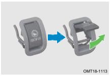
Step 2: Turn up the plastic cover to access the anchorages;
