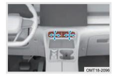
Move center outlet adjustment lever up and down, left and right by hand to adjust direction of airflow.
