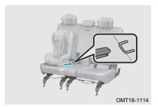
Step 3: Place the child restraint system on the rear outboard seat;
