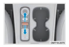
Dial the button upward to increase the volume and dial the button downward to decrease the volume.
