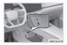
Front USB is located on the lower part of auxiliary fascia console (as shown in the illustration).
