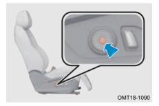
When the vehicle is powered on, press the massage function switch, the audio system pops up the seat control screen while the massage function is turned on.
