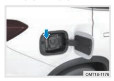
The charging/discharging indicator is located in charging port cover. Indicate the charging/discharging status in yellow, green, blue, and red respectively.
