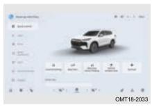
When the vehicle is powered on, click " " button through Audio System - Settings - Quick Control to unlock/lock doors.
