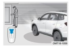
ON: Turn vehicle power to OFF mode, turn on headlight automatic mode before stopping. When the vehicle is in a dim environment, press lock button on smart key, and the vehicle is armed successfully. Low beam lights automatically come on for tens of seconds. Press lock button on smart key to activate it again.
