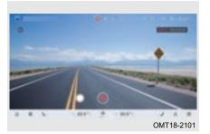
The driving recorder is connected to the audio system through Wi-Fi and is displayed and operated on the audio system. Click driving recorder application to enter the real-time screen of it.
