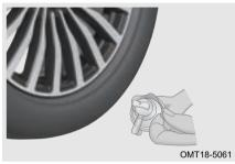
Shake the automatic inflation tire repair liquid well before use, and then tear off the safety belt of the junction valve;
