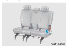
Pull the seatback adjustment lever upwards, adjust the seatback to desired angle, and release the lever to adjust the seatback angle.
