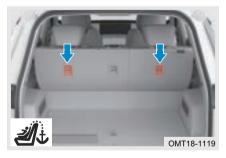
This model is equipped with top tether strap anchorages on the back of the rear seats.
