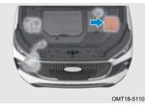
Remove the engine compartment fuse and relay box cover to inspect or replace the fuse.
