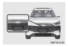
Installation position of front camera: Lower middle part of the front license plate.
