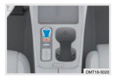
Press hazard light switch to turn on and press it again to turn off.
