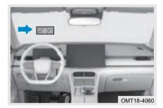
The head up display is located in the front windshield area.
